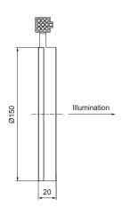
Cable permitted bending radius: 43.2 mm
