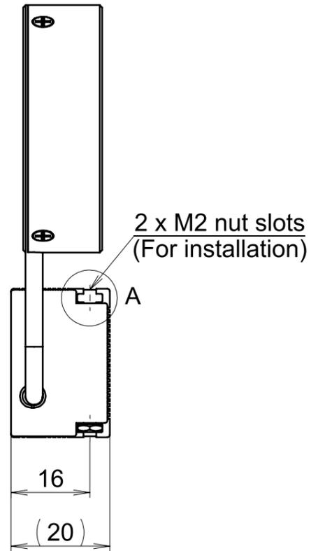
Nut slot detail diagram
