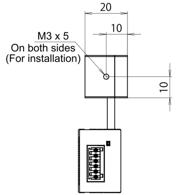
Nut slot detail diagram
