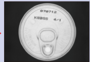
With the LFX2, the output is sufficient for proper imaging at a shutter speed of 1/4,000.
